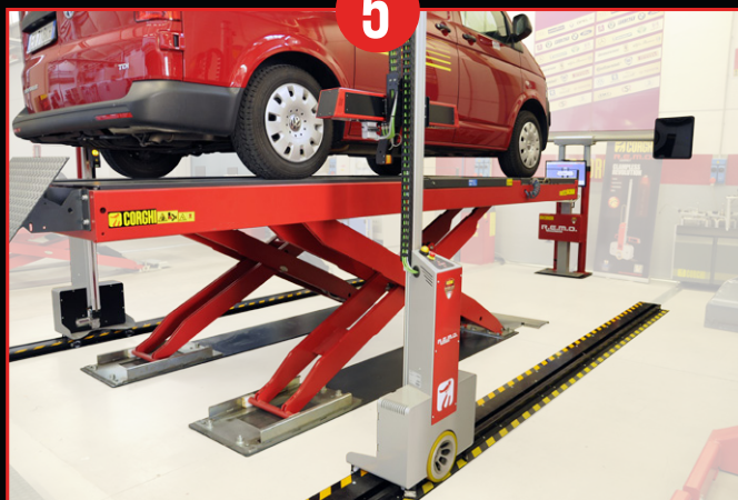
Possibility of reading even when the lift is raised
