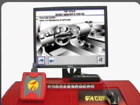
**CAL ONE-TOUCH**, steering wheel rotation sensor calibration system integrated in the wheel aligner. Essential for correctly aligning wheels on cars equipped with ESP, adaptive suspensions, dynamic steering, electric power assisted steering and adaptive lighting systems.
