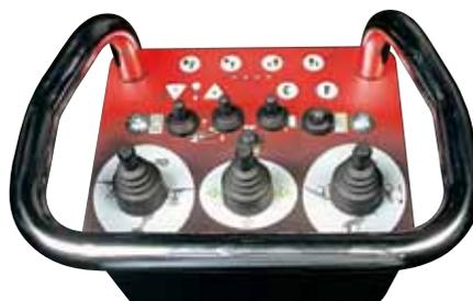
The **new manipulator** with **ergonomic** controls ensures the tyre changer's complete functionality, with no need for the operator to **come into contact with the tools**.
